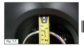
(f) Confirm the alignment of the tip to ensure the gap from the top of the tip to the fascia is  $25 \pm -5$  mm (Fig. 3-5).
